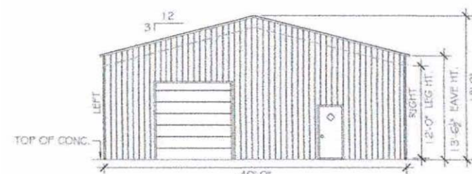
FRONT END WALL ELEVATION SCALE: 3/32" = 1'
