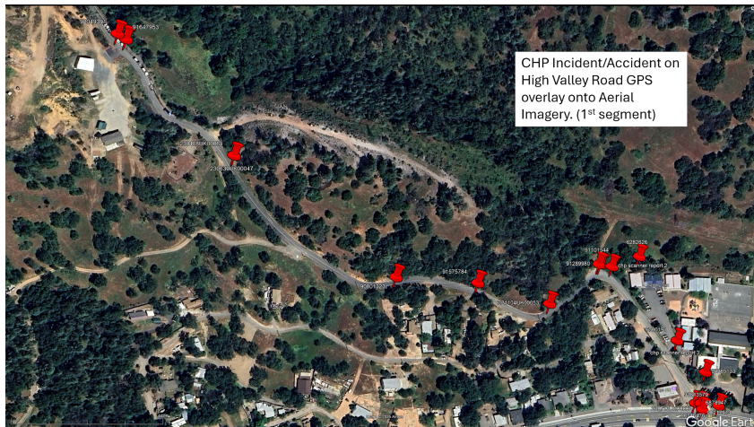
Figure E2a: High Valley Road CHP Incidents and Accident overlay onto Aerial Imagery. Note: clusters of accidents where road is not compliant for curve radius (near school) and road width (along hillside).
