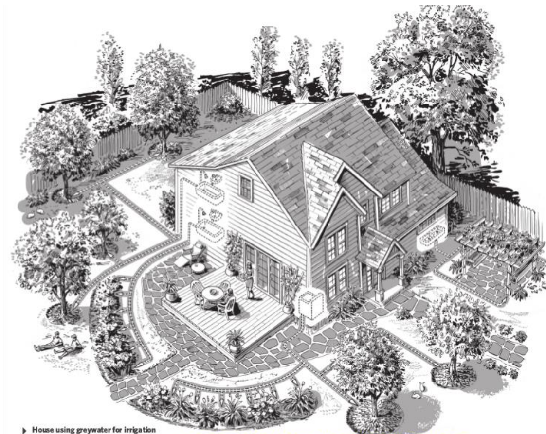
► House using greywater for irrigation with simple laundry-to-landscape and branched-drain systems
