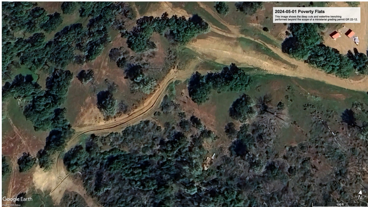
Figure B7: Shows deep trenching for waterlines and deep cuts and bench into steeply sloped land.
