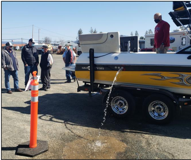
Figure 6a. March 2021 refresher for Clear Lake Ramp Monitor Crew of a wake boat. Here the crew sees the remaining water in a ballast tank after the pumps shuts off; furthering the need for thorough inspections.
