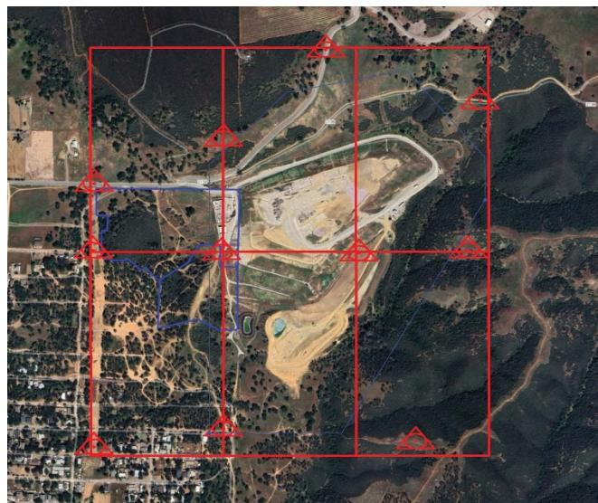
SHN will survey the area and provide a topographic map with a contour interval of 1-foot, and orthographic photo. The cost for this task includes all site visits (7 total) required to verify aerial target controls, set control points and aerial targets, and supplemental ground surveys. All aerial data will be compiled into a topographic survey compatible for use with AutoCAD Civil 3D.
