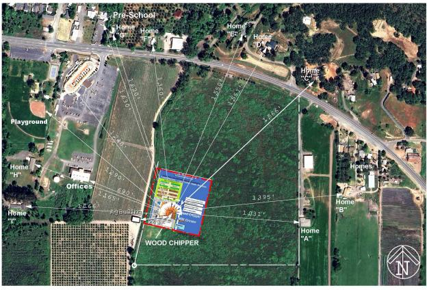
FIGURE C - DISTANCES FROM NOISE SENSITIVE RECEPTORS TO WOOD CHIPPER NOISE
