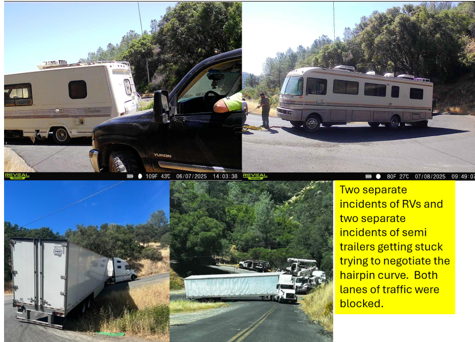
Figure E5b: Photos of vehicles blocking traffic for extended periods that became stuck while trying to negotiate the hairpin curve on HighValley Road.
