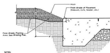
Growing shall provide for natural runoff of water without low spots or pockets.
