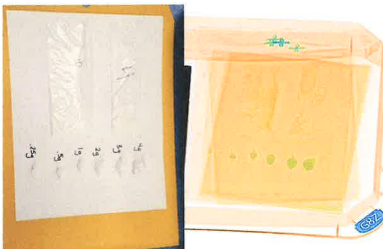
Figure 8: Optional X-Ray system provides visualization of various amounts of powders contained in 170 sheets of paper.
