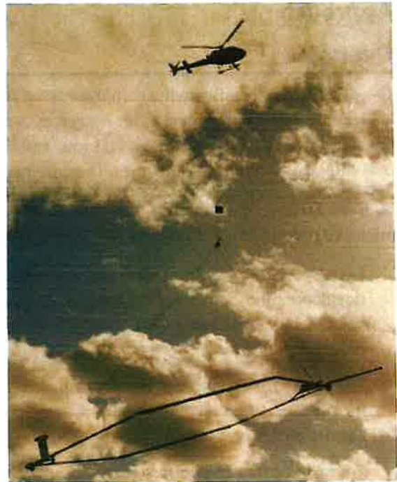
The SkyTEM system in operation during a recent AEM survey conducted in California
