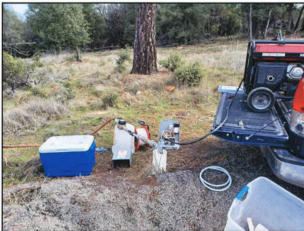
Photo 1: View of site well during well yield test.
