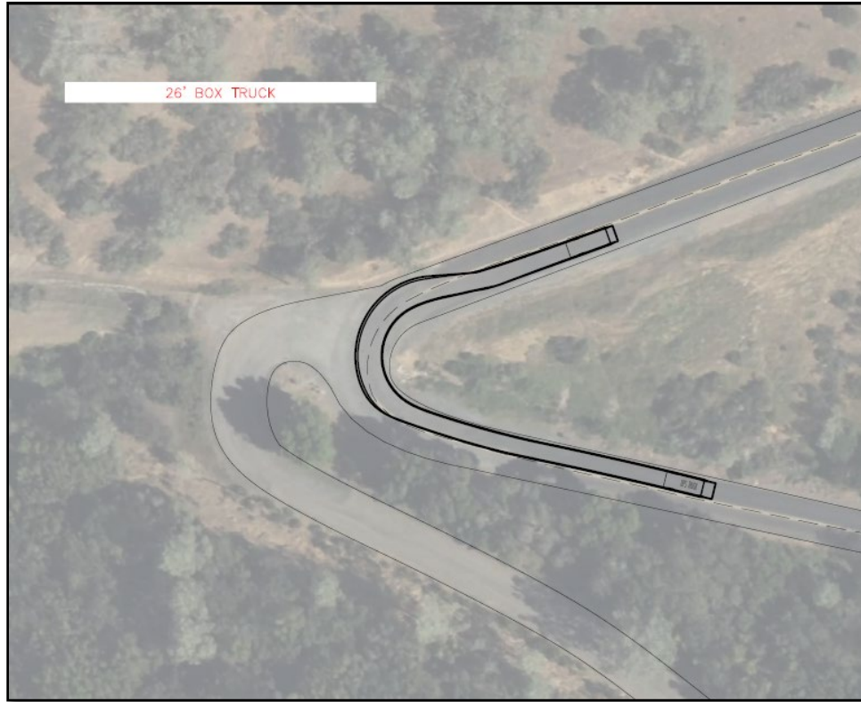
Figure 4. Turning Radius - 26' Box Truck
