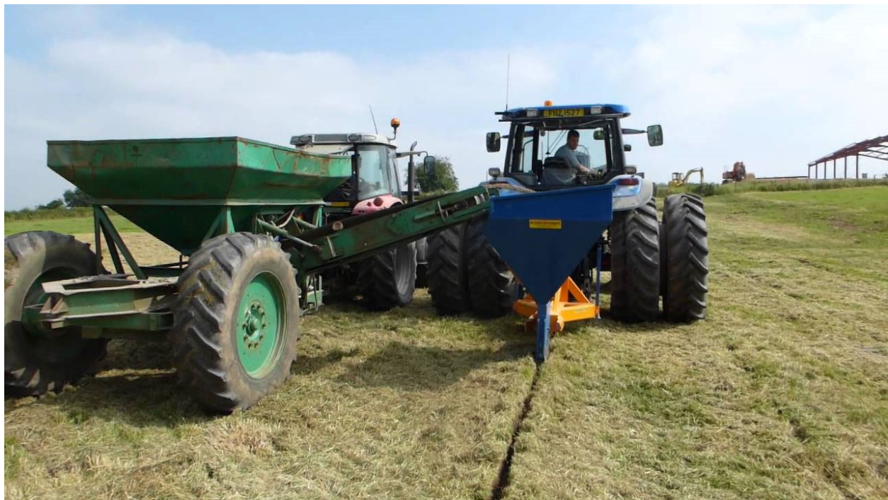
Mole drain installation setup with mole plough and hopper for gravel backfill
