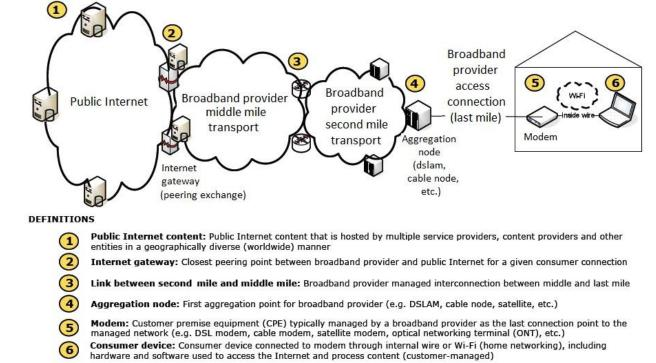
Figure 20. Basic network structure from the FCC's Broadband Availability Gap Paper
