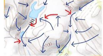
map represent existing swales that were constructed to effectively manage all storm water runoff in this area which has historically been used for small-scale agriculture. These existing swales guide the flow of the storm water runoff through rocks and vegetation to either disperse over vegetated areas or to ultimately join with the natural channels for storm water runoff. These rocks and vegetation afford a natural filtration for the mobilized sediment in the stormwater sheet flow.
