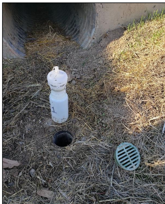
Figure 3 Example of in-ground storm water sample bottle located directly outside an urban discharge source.
